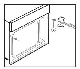
■ Push the appliance into the niche. After aligning the oven it must be secured in position. Open the oven door and using the two supplied screws ⑨, secure it to the cabinet through the holes on either side of the vertical oven trim.
