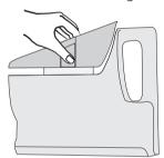
■ Remove the insert by pressing the handles together and lift upwards at an angle.
