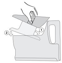
■ Reinsert the insert into the steam generator only when both parts are dry. Place the insert in at an angle ① and lower the side with the opening ②.
