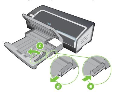
f Reload the desired media into the output tray (see Loading media in the input tray).
