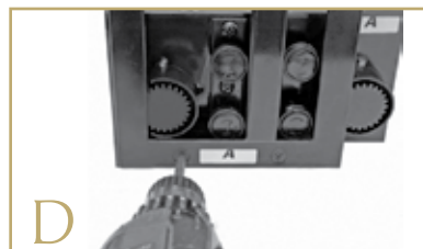
Secure Side rail A using 2 screws. Repeat for Side rail B
