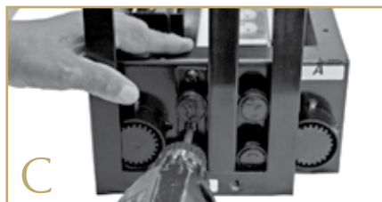
Secure roller attachment using 2 screws
