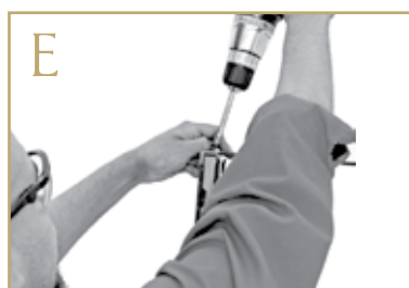
Attach safety bar to top of unit using two screws.
