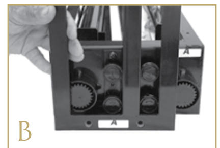
Position side rail A lining up the gear rack over the spur gears
