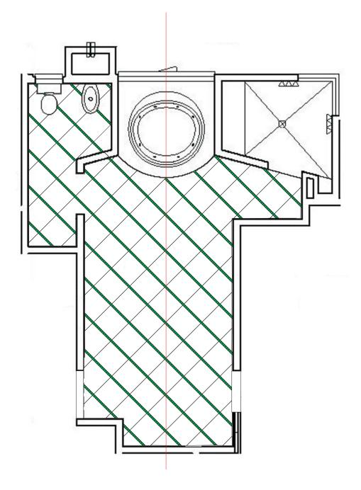
Torreon Stone 24x24 at 45 degrees Rain Forest 2"x2" sq on one diagonal Torreon Stone rectangular threshold at bed room and at closet
